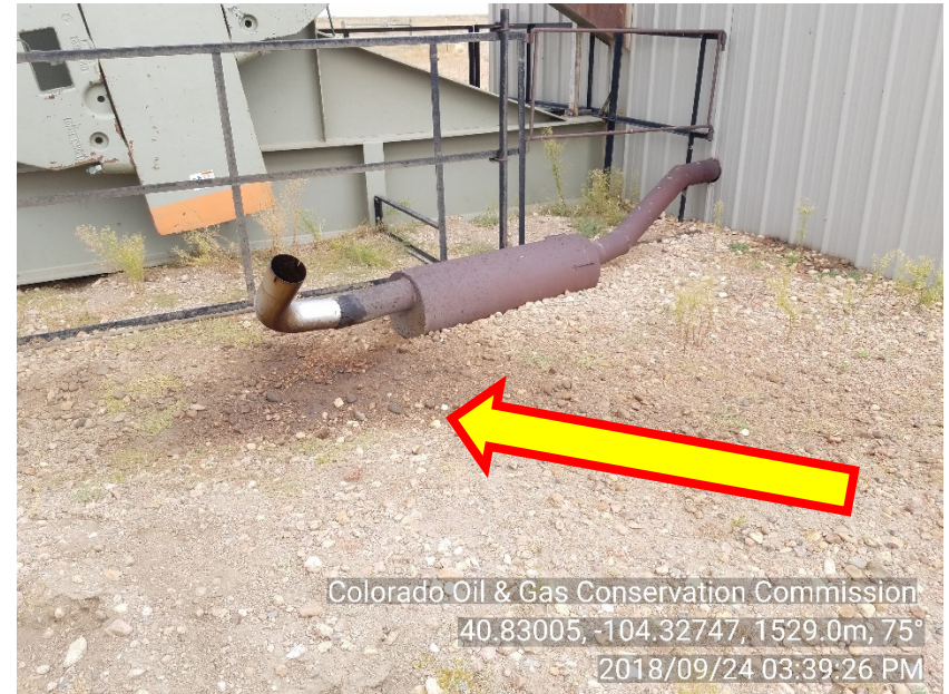
Photo #6 Smuggler 16-10-62 engine exhaust Stained soil
