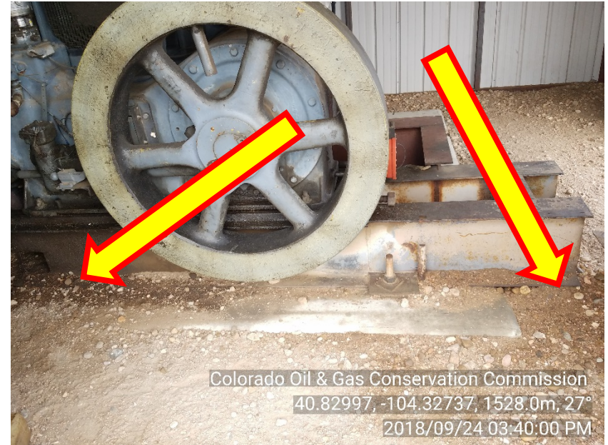
Photo #4 Smuggler 16-10-62 gas engine Stained soil
