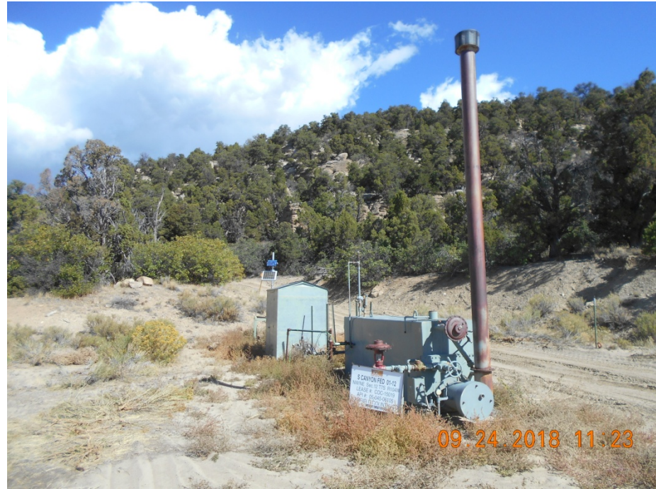
Separator Meter housing with sign. Weeds around fired equipment.
