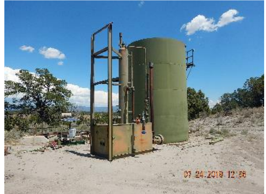
Photo 6: Production tank and separator stored on location.
