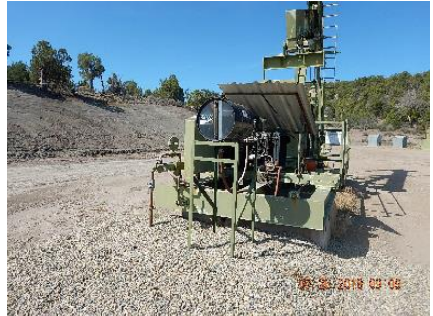
Photo 8: Lube oil tank with no spill prevention.
