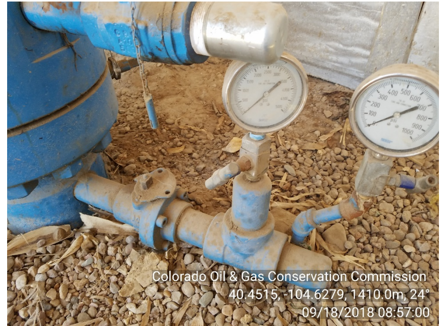
Casing and surface casing pressure gauges
