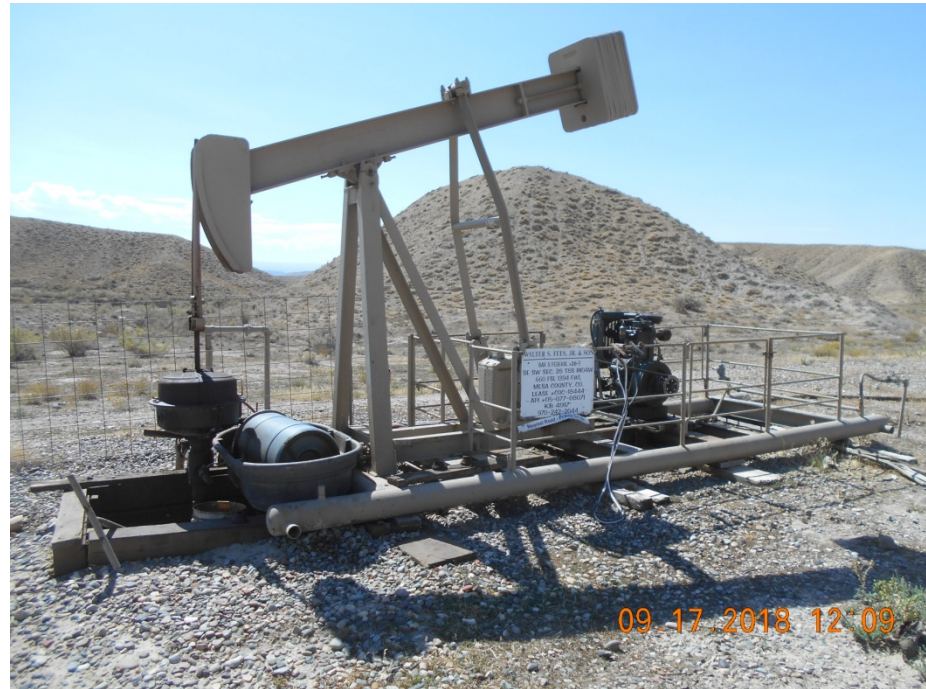
Wellhead with pump jack
