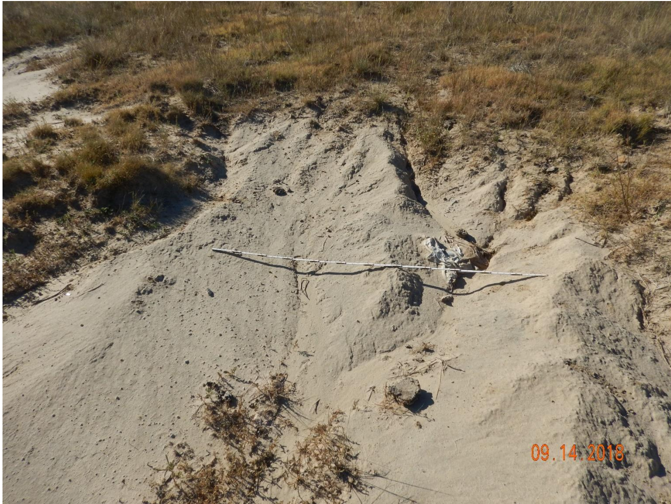
Photo 5: Continued from photo 4. Photo shows erosion degradation occurring on location. 6 foot measuring stick for reference.
