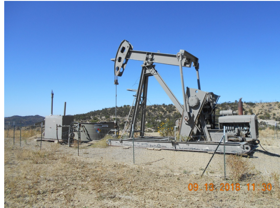
Pump jack, Separator, Tank battery
