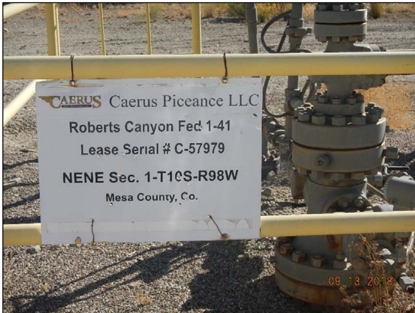
Photo 1: Wellhead sign missing access road and emergency contact info.
