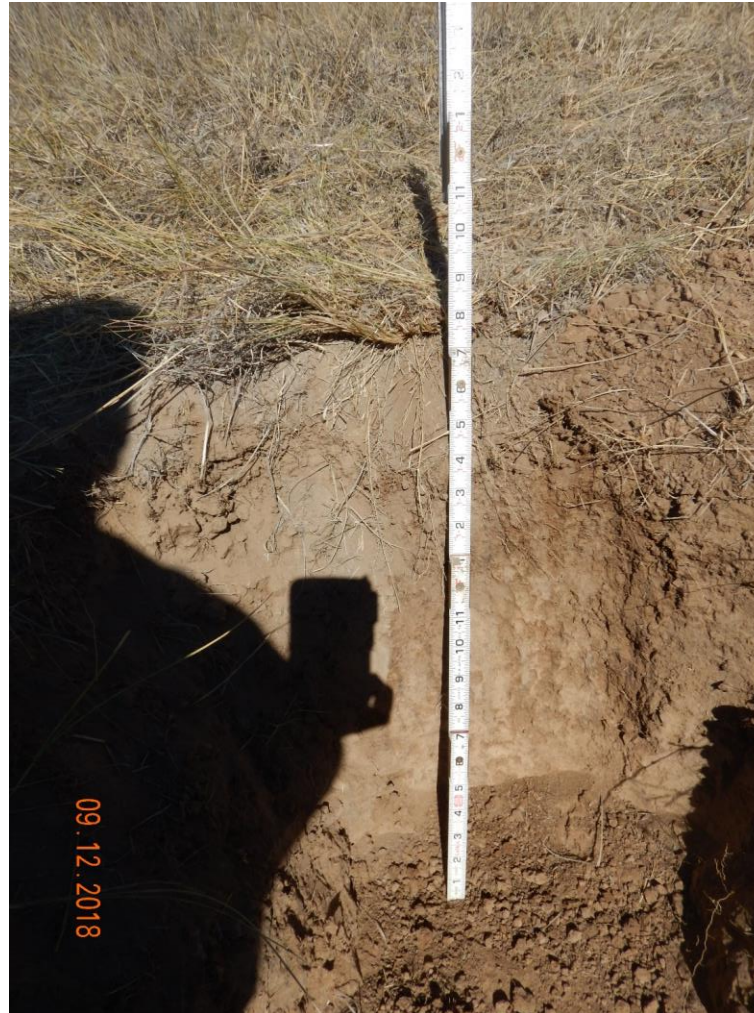
Photo 17: Photo taken from the west of the pad on adjacent to the disturbance. Contractor on site indicated that "~8 inches of topsoil" is being salvaged and stored on the east end of the location". Contractor indicated that he was unaware of the actual depth of the topsoil horizon. Photo shows that it appears that the topsoil horizon exceeds 8 inches in depth.
