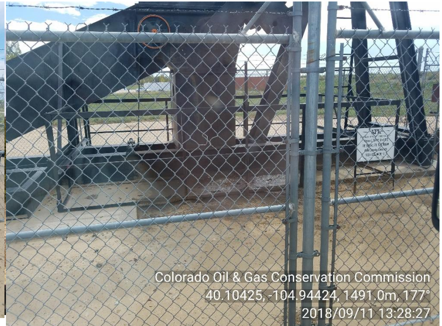
Photo 2. Fluid leaking from pumpjack gear box
