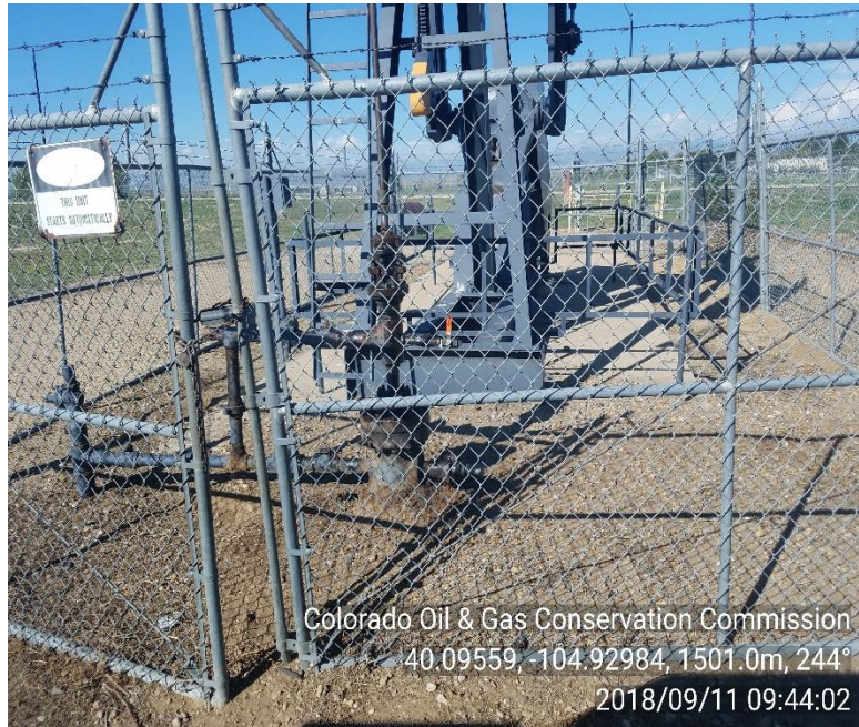
Photo 3. Faulty equipment/stained soil
