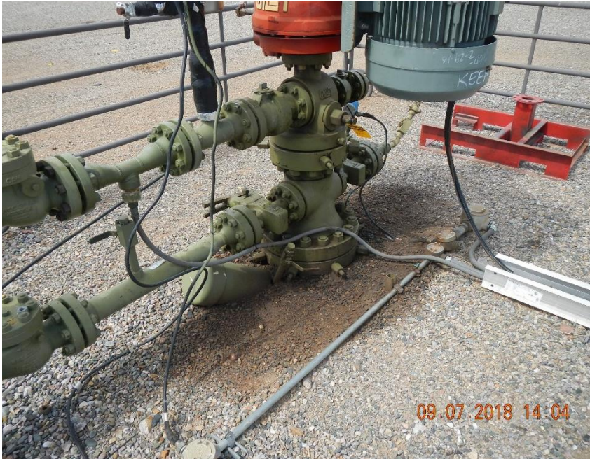
Oil stained soil below pump.
