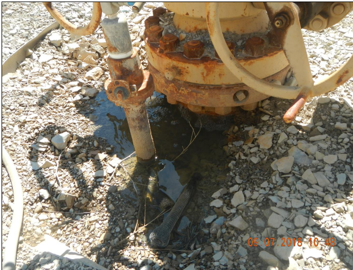
Gas bubbling around well surface casing. Shell 697-34-05
