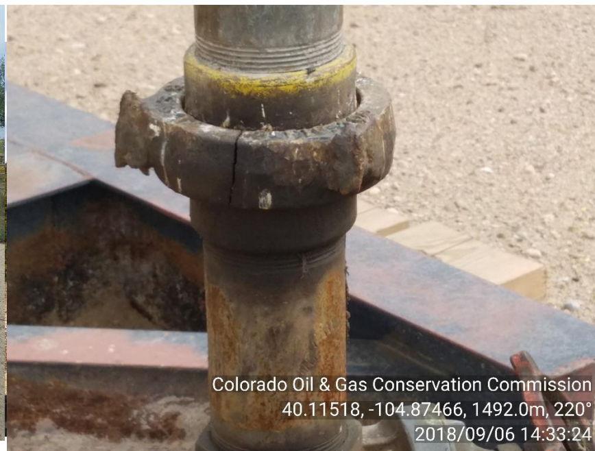
Photo 2. Cracked hammer union in plug above master valve
