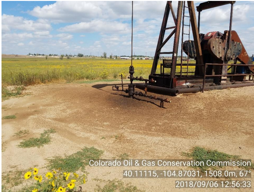
Photo 1. Wellhead/Stained soil around wellhead all the way into the weeds to the North
