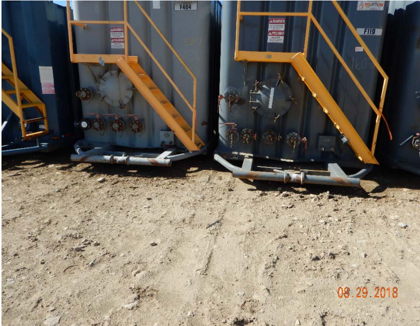
Photo #3 – Frac tanks stored on location lacked secondary containment devices on inspection date.
