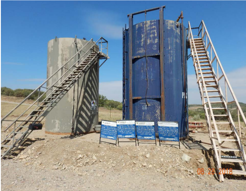
Photo #1 – Well signs on south side of temporary tank battery. Note inadequate berm construction.
