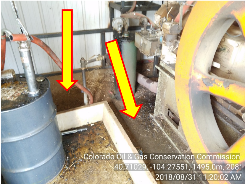
Photo #11 Joker 36-9-62 Engine house Stained soil & engine base
