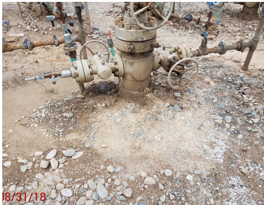
Location Photo #5, stained soil under valve
