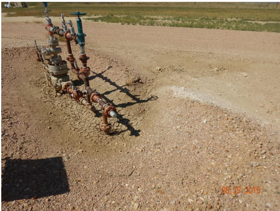
Photo 11: Photo taken from the wells, photo shows berm at well no longer in proper functioning condition.
