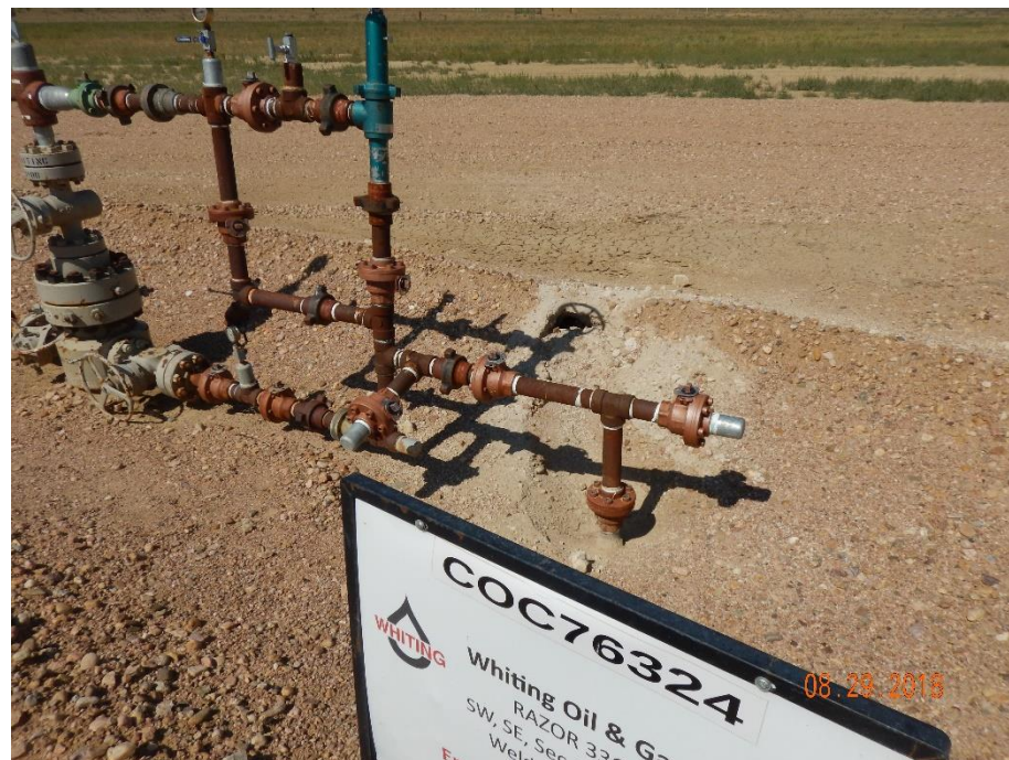
Photo 12: Photo taken from the wells, photo shows berm at well no longer in proper functioning condition.
