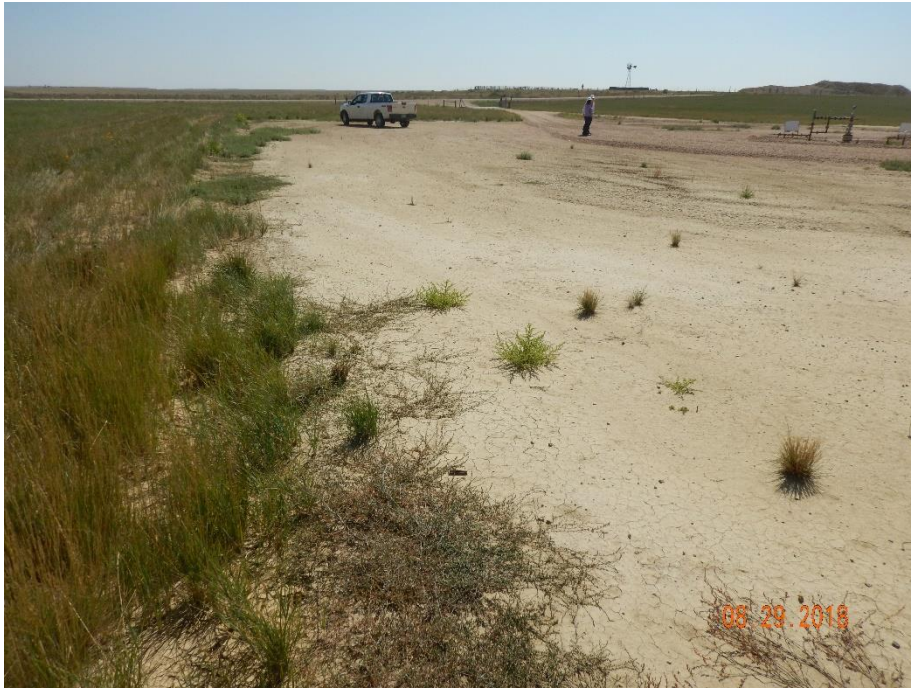
Photo 9: Photo taken from the northeast end of the location, facing south. Photo shows areas around the wells that do not appear to be reasonably needed for production activities do not appear to have been reclaimed or stabilized.
