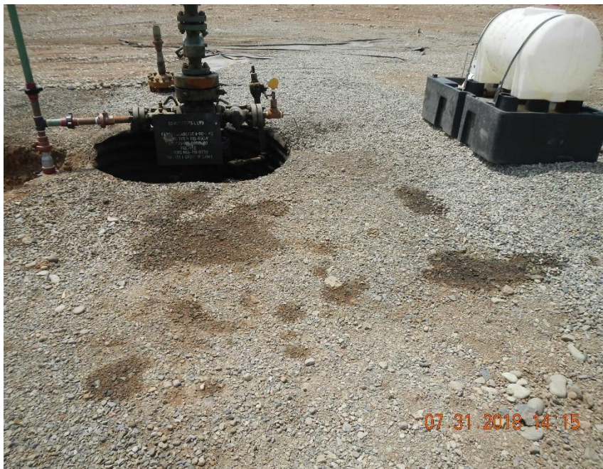
Stained soil near well head.
