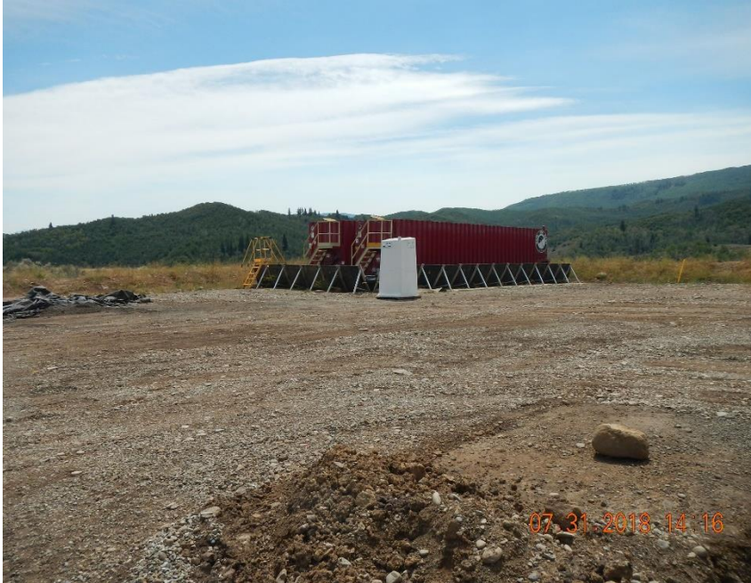
Frac tanks used for drilling fluid during drilling operations.
