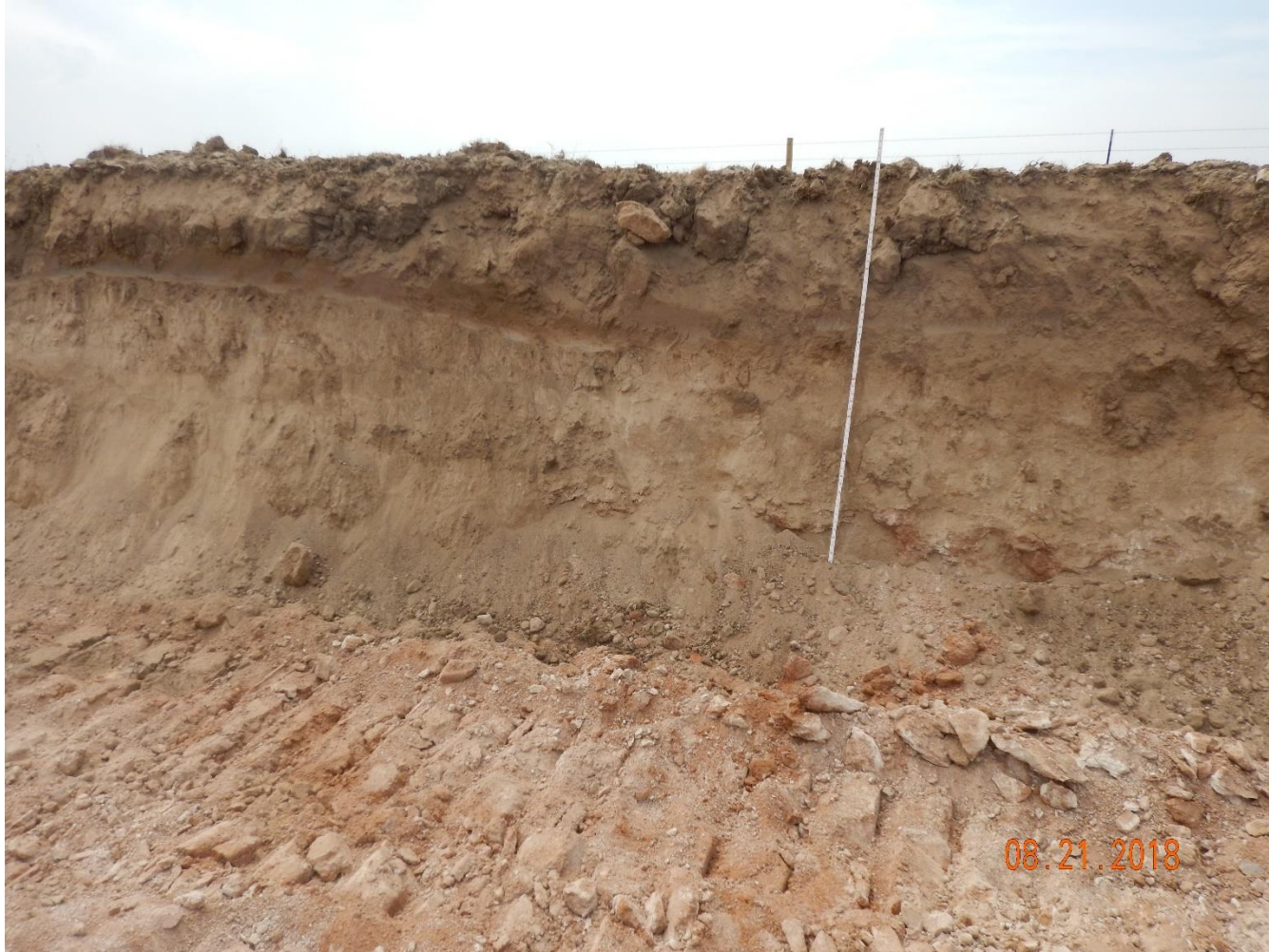
Photo 3: Photo taken from the south end of the location, facing south. Photo shows soil horizons from the cut. Topsoil layer appears to be ~2 feet in depth from surface.
