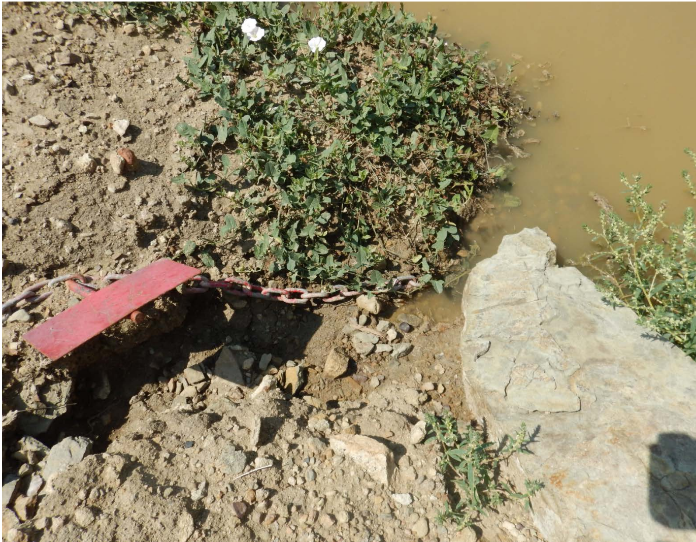
Freeboard level marker is partially submerged
