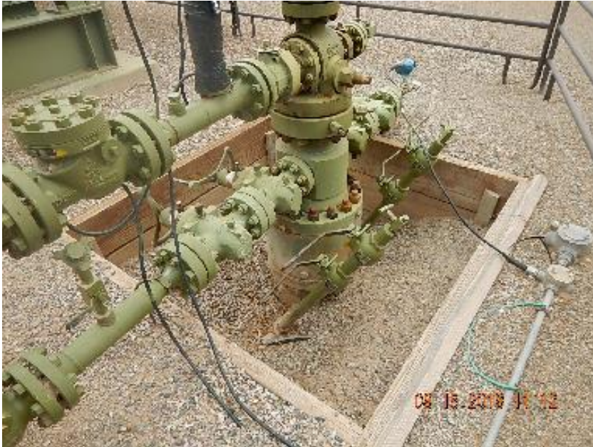
Photo 9: Open wellhead cellar.
