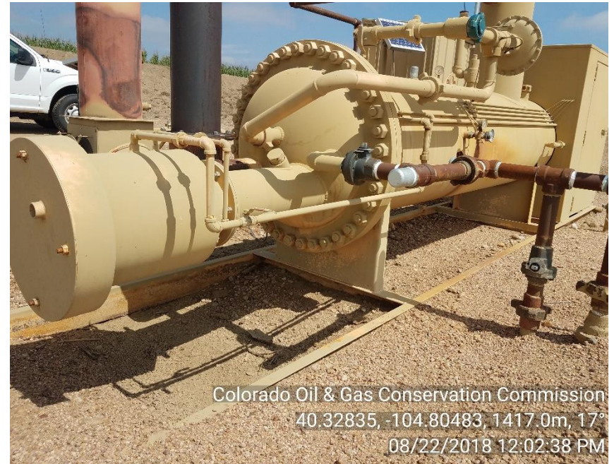
Separator is not anchored.
