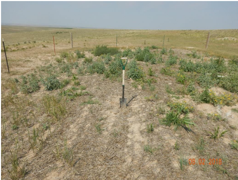
Photo 11: Photo taken from the fenced area of the well, facing west. Photo shows compaction alleviation and revegetation activities appear to have been conducted in the area of the well. Inspector was able to easily penetrate the top 8-10 inches of the soil with a shovel.
