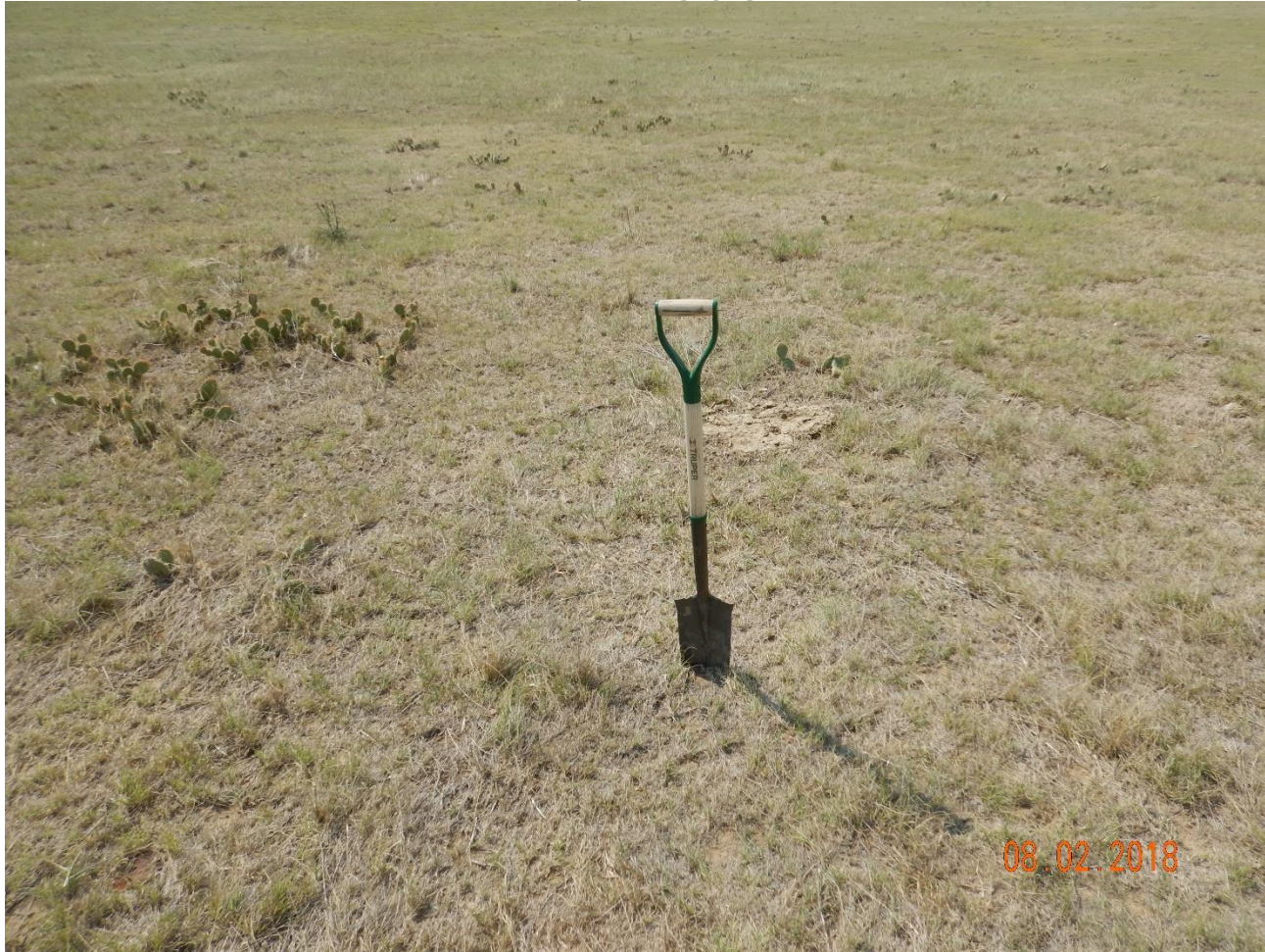
Photo 13: Photo taken from the adjacent reference area. Photo shows inspector tested the soils in the reference area for compaction to compare to the disturbed areas of the location. Inspector was able to easily penetrate the top 8-10 inches of the soil with a shovel.
