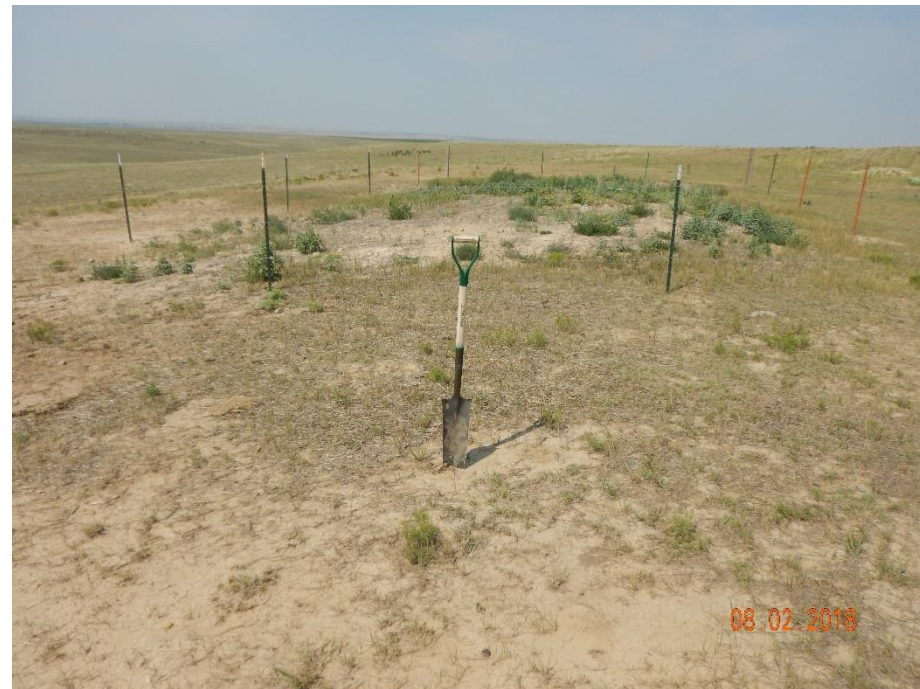
Photo 12: Photo taken from outside of the fenced area of the well, facing west. Photo shows compaction alleviation and revegetation activities DO NOT appear to have been conducted in the remaining location. Inspector was able to penetrate the top couple of inches of the soil with a shovel; compaction concerns evident.
