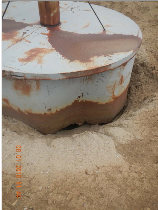
Photo 5. Hole in tank bottom.
