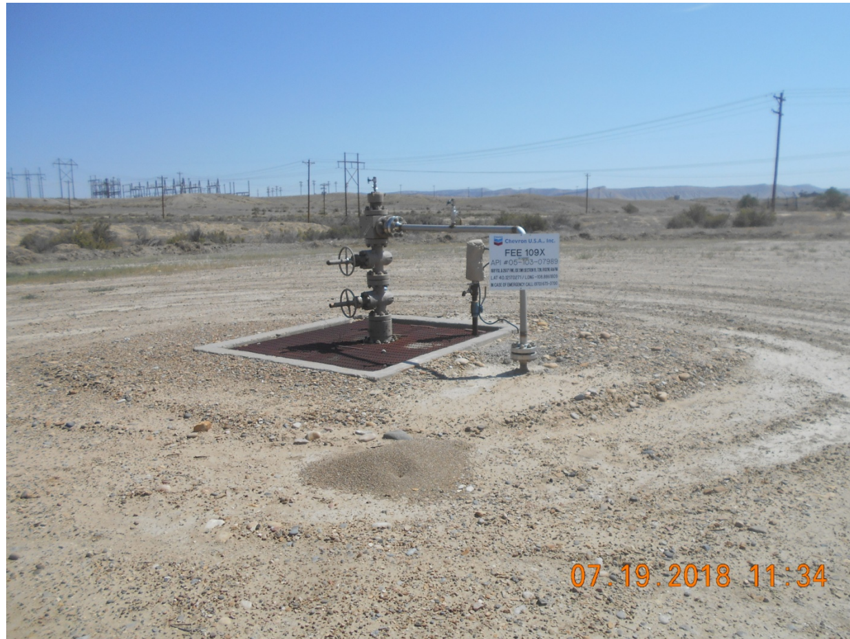
Injection Wellhead
