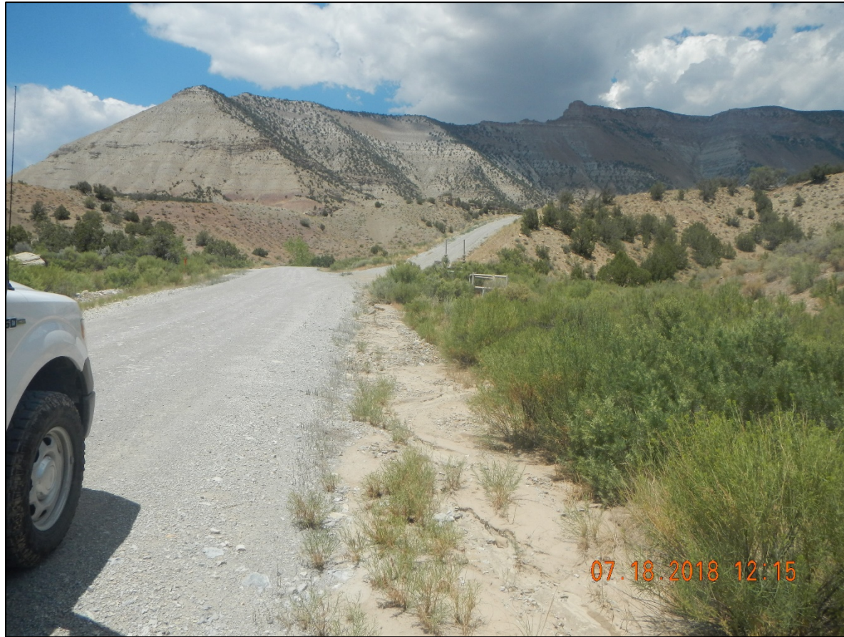
Sediment in ditch on main road just before access road. 39.47601 -108.06135
