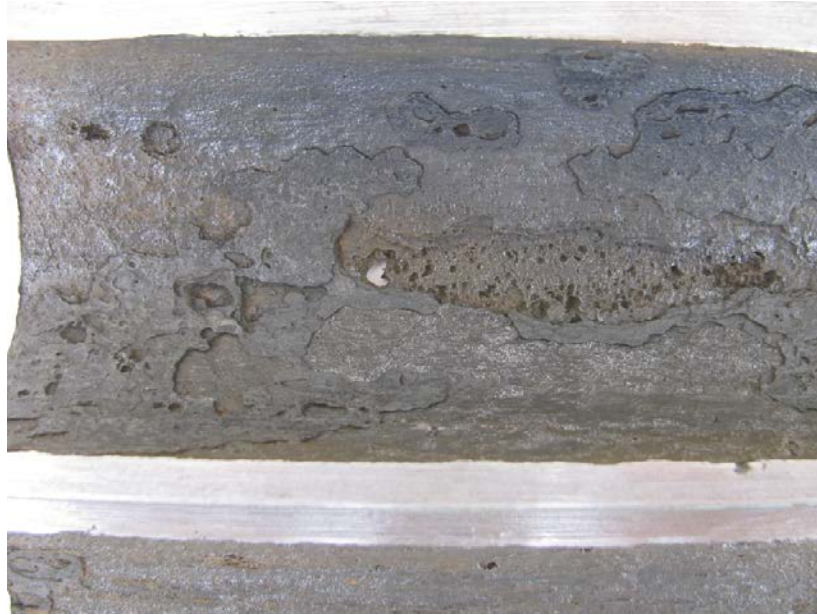
Photo # 4. Close-up of top section, heavily pitted with through-wall hole
