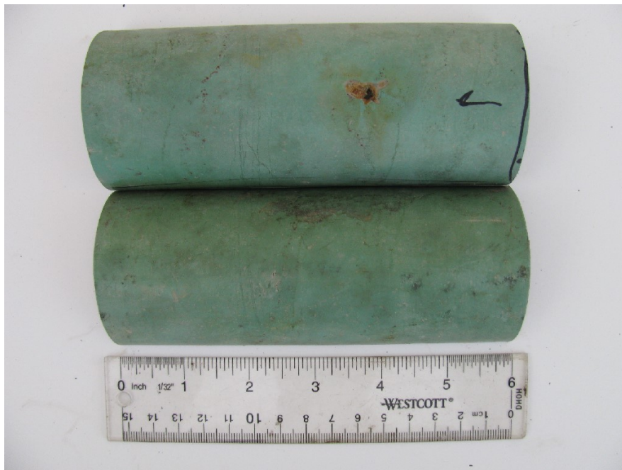
Photo # 1. Cut and split section of flowline with failure, exterior view
