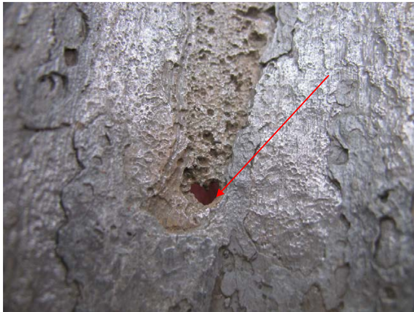
Photo # 5. Through-wall hole noted with red arrow
