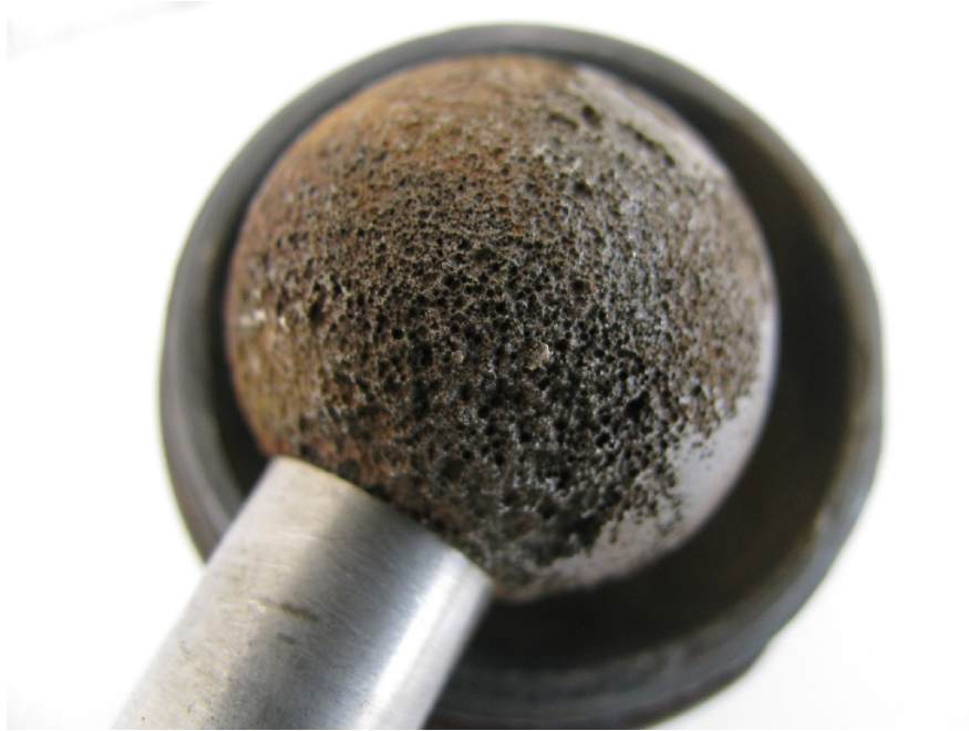
Photo # 7. Corrosion damage on the stem
