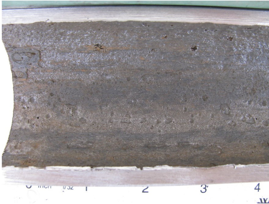
Photo # 6. Lower section of flowline cut-out with light pitting
