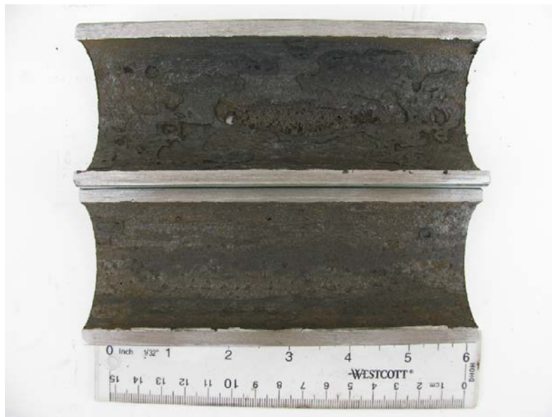
Photo # 3. Cut and split flowline with through-wall hole (upper half)
