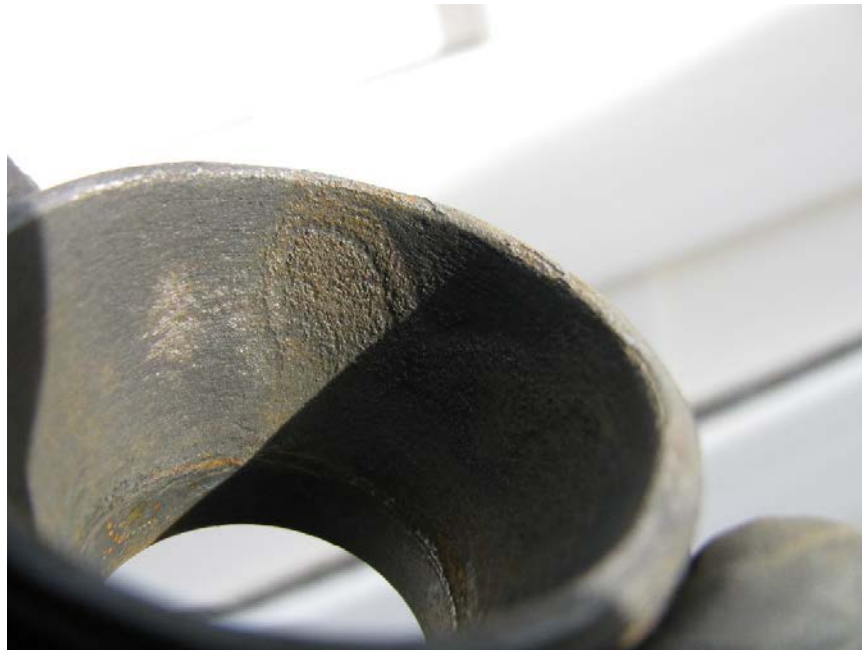
Photo # 8. Corrosion damage on the seat
