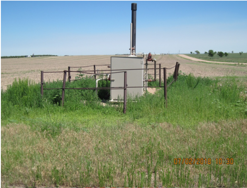
3. Horizontal heater treater
