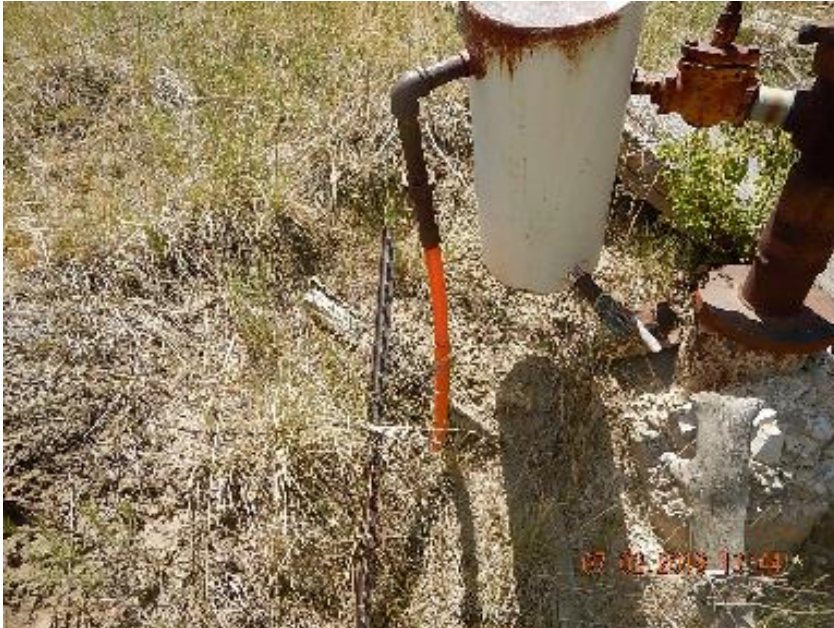
Photo 5: Flow line off knock out.
