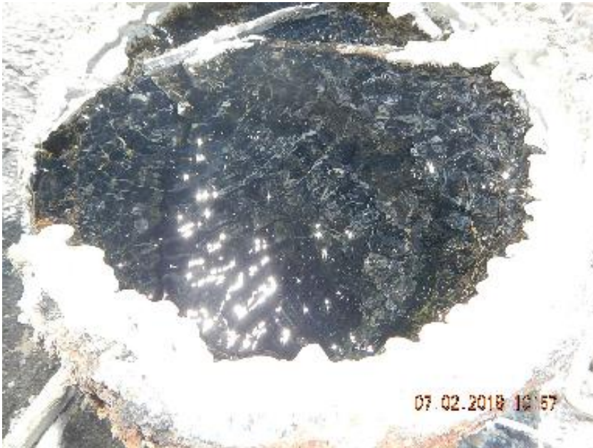
Photo 5: Close up of casing with possible intermediate casing shadowed in fluid. Flow off left side of casing.
