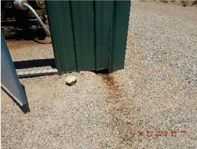
Photo 3: Impacted soil and gravel at exhaust outlet.
