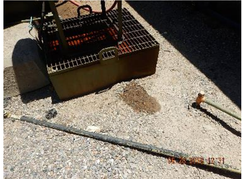
Photo 4: Impacted soil and gravel at lube oil tank spill prevention.
