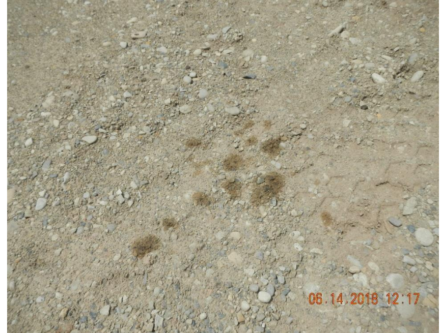
Lube/hydraulic oil leaks on pad.
