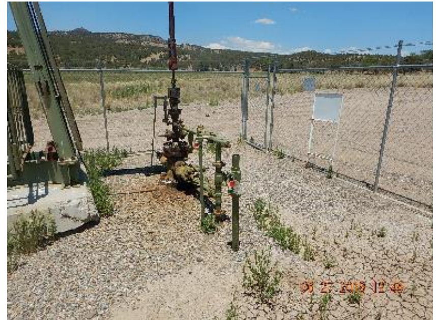
Photo 2: Unused risers at wellhead and impacted soil and gravel at wellhead base.
