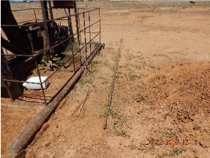
Photo 5: Sucker rod and production related debris at pump jack.
