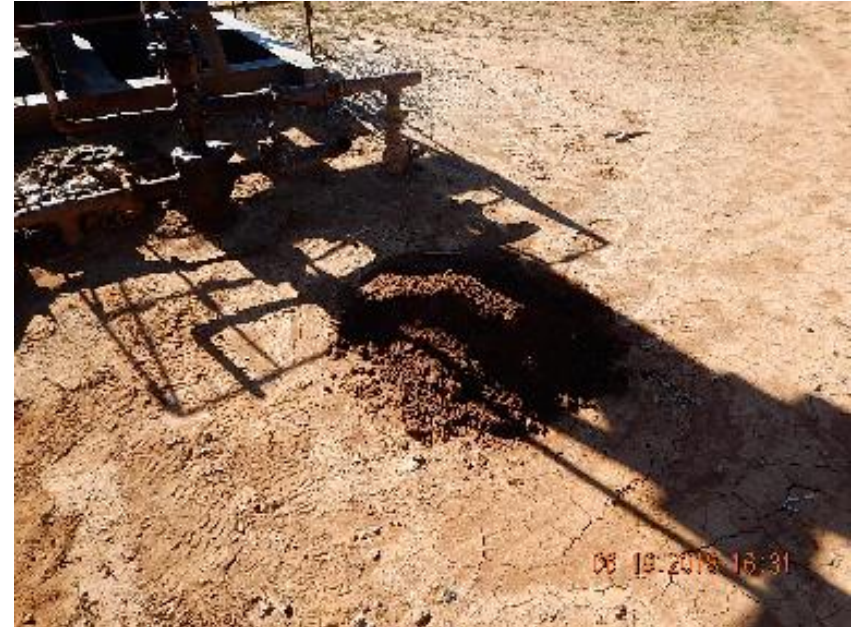
Photo 4: Impacted soil at wellhead..
