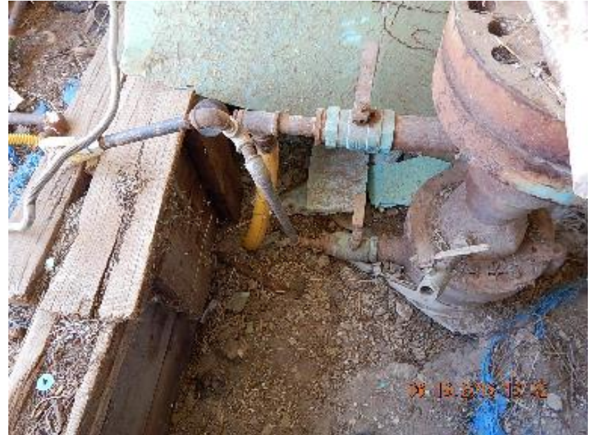
Photo 6: Yellow poly line off wellhead casing.
