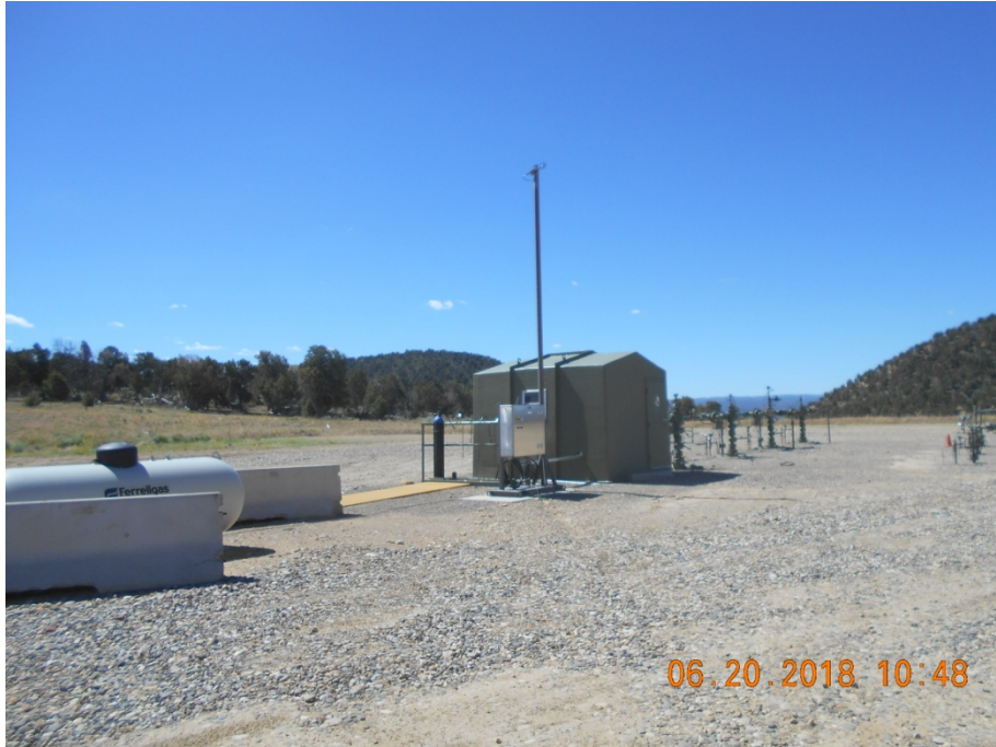
Injection wellhead housing
