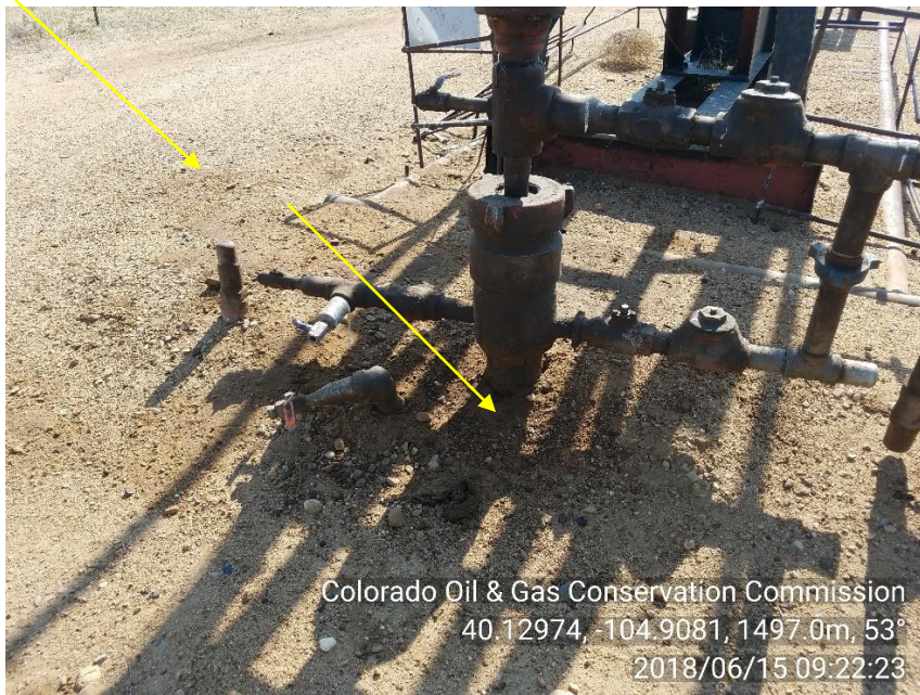
Photo 3. Stained soil around wellhead and fanning out to the northwest.
