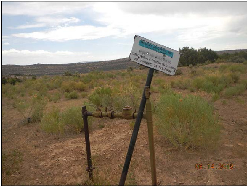
Photo 1. Wellhead next to riser. Sign missing public road used to access the site.
