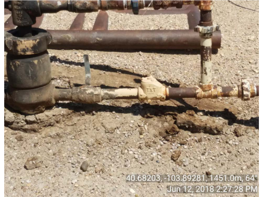
Photo 3: Stained soil at wellhead.
