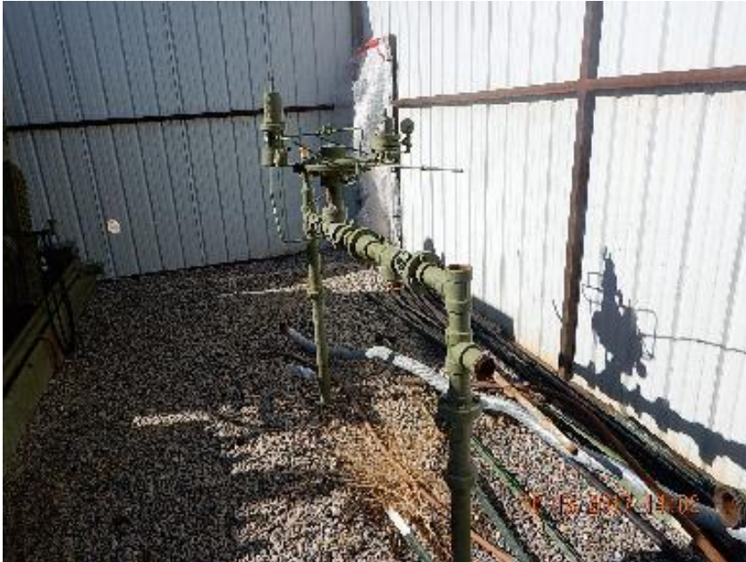
Photo 3: Unused riser with open ended pipe previous inspection.
