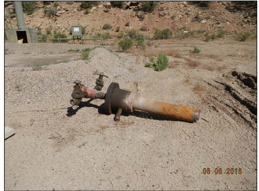
Photo 2. Cut off wellhead stored near tank containment.
