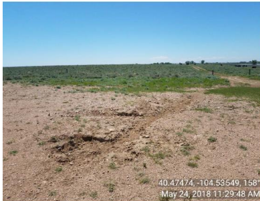
Photo 4: Stormwater erosion at SW corner of location.
