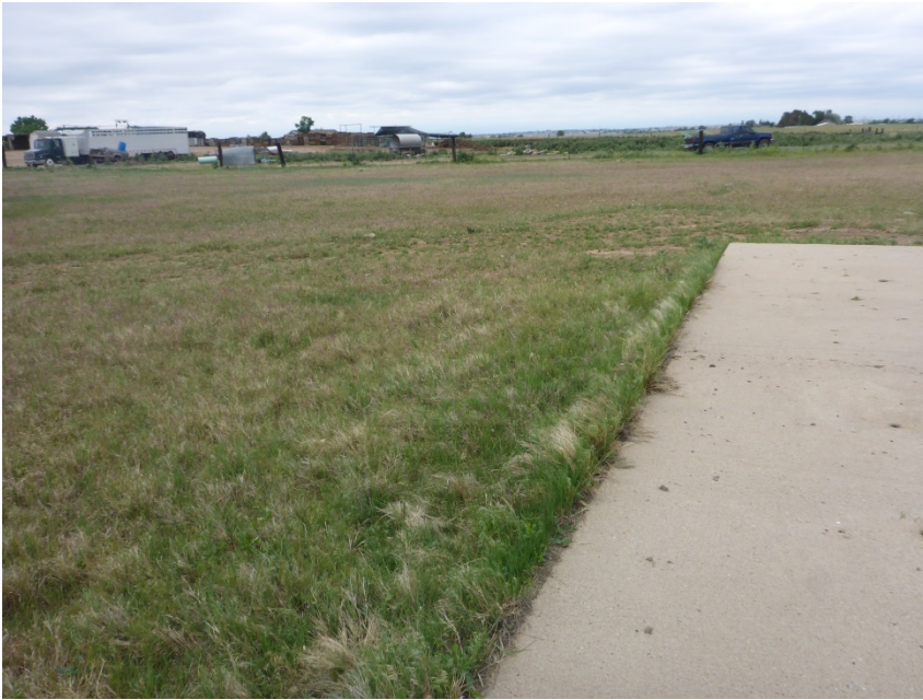
Photo 1. Photo taken from the location, facing West. Appears the Operator has performed final reclamation activities at the well site and access road to the facility. The concrete slab was left on location.
