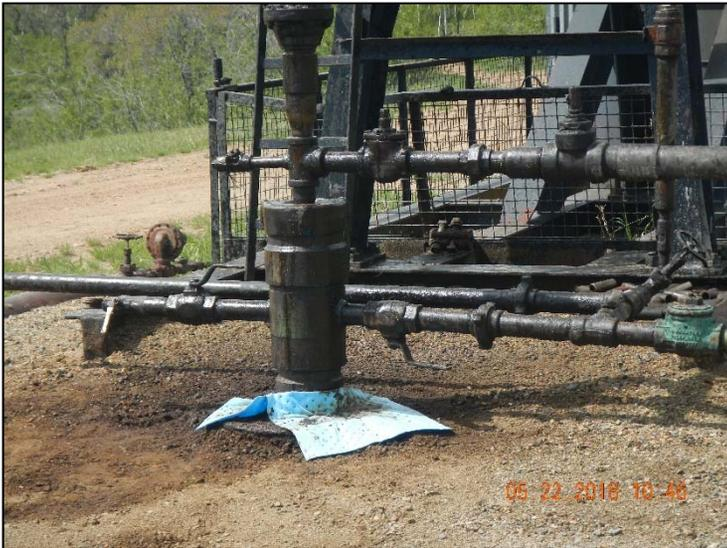
Photo 4. Close-up of wellhead and absorbent pads.
