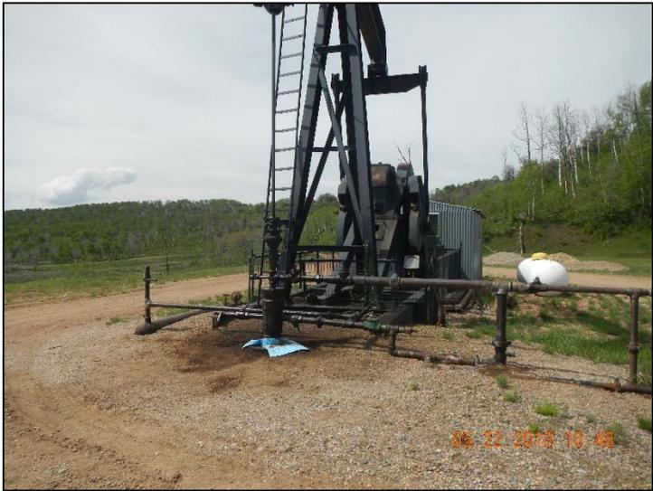
Photo 3. Stained soil and absorbent pads at wellhead.
