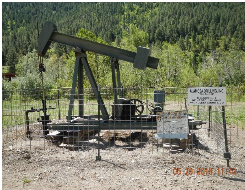
Nielson #4 well head and electric pump jack.
