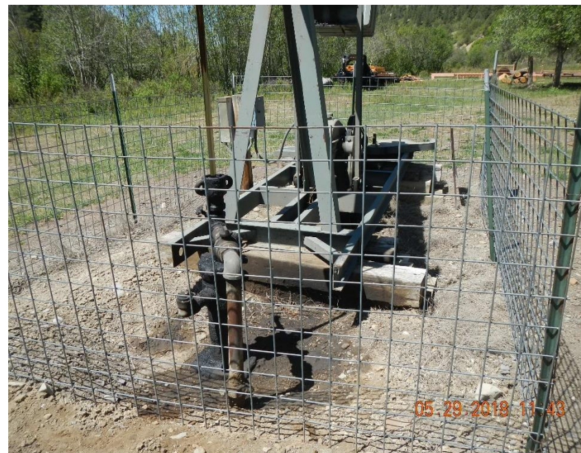
Stained soil at well head. Noted on previous inspection.
