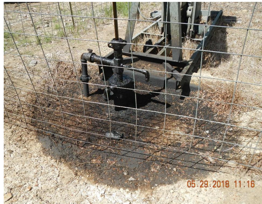
Stained soil around wet well head, noted in previous inspection report.
