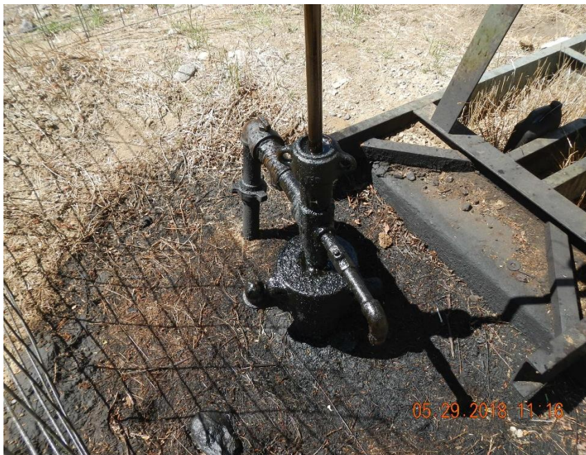
Well head is wet with oil. Area surrounding well head is stained.
